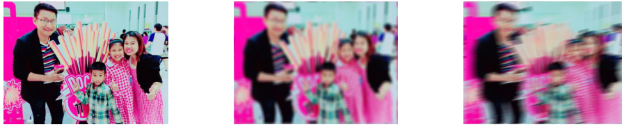
Figure 3.2.6: Data used in numerical experiments. The true RGB image of size 336 \times 252 \times 3 , Degraded image with Gaussian blur of size 9 \times 9 and \sigma = 4 and the motion blur image with \text{len} = 21 and \theta = 11 .
