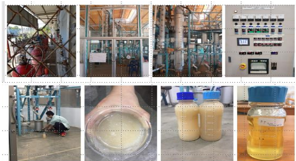
Figure 54 FT–Synthesis Apparatus and Yields from the FT Process
