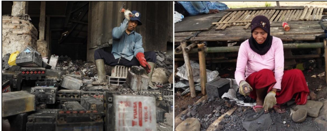
Figure 39 A man and woman in Tegal, Indonesia use hammers to break up used lead–acid batteries for recycling [from 150]
